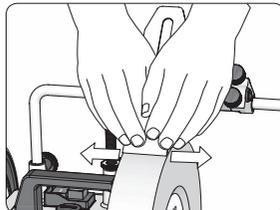
*Grind again with a light pressure on the graded stone. The plane iron remains in the same position in the jig.*
