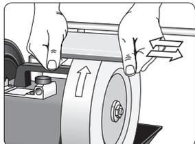
*Press the coarse side of the Stone Grader onto the stone for 20–30 seconds while moving it sideways across the stone. The stone has now returned to normal fast grinding.*
