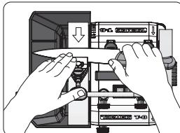
**3.** The universal support is now set to the right height for the desired angle of the knife in the knife jig, and you can start sharpening your knife. The KS-123 Knife Angle Setter is self-adjusting for the grinding wheel diameter.
