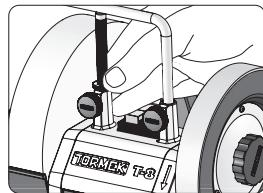
3. Lower the universal support slightly lower than you think you will need, as it will be easier to adjust the angle by raising the universal support. Leave the knobs on the universal support loosened.
