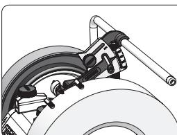
The three reference legs (5.) should rest over the grinding wheel, but don't have to all be in contact with the grinding wheel in this position.
