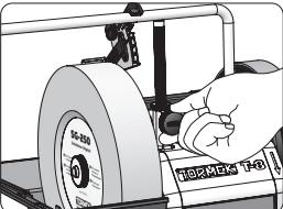
**2.** After raising the universal support so that the angle indicator points to the desired sharpening angle, lock the universal support knobs and remove the KS-123 Knife Angle Setter from the universal support.
