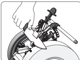
Insert the knife blade with the edge **centered** in the V-shaped edge rest (6.) with the knife jig on the **right** side of the angle setter.
