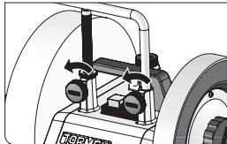
2. Make sure the knob for locking protusion (7.) and the two knobs on the universal support mounts are loosened.
