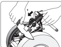
Slide the knife forward, along with the retractable part (1.) and set the stop of the knife jig against the universal support.
