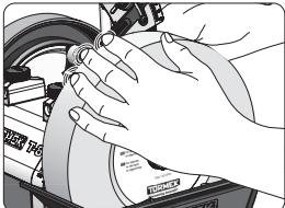
**1.** Put one finger on each of the three reference legs (5.) with a light pressure. Raise the universal support until the angle indicator (4.) points to the desired sharpening angle on the angle scale (3.). Make sure that all three horizontal legs are resting against the grinding wheel in this step.
