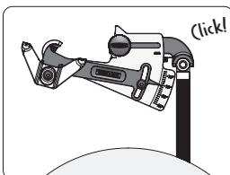
Attach the KS-123 Knife Angle Setter to the universal support by snapping the holder for the universal support (2.) into place.
