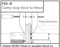
fence to stop Right Angle Fixture before bit contacts wooden runner.
