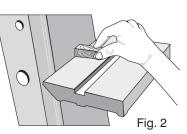
into the tubes (FIG. 2). If any excess glue remains inside the tubes it should be gently scraped out.
