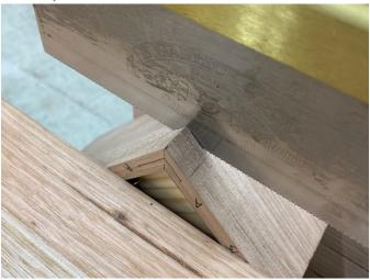
Cut commercial veneer stock into little triangles roughly 25mm x 25mm. You will need a minimum of 8 of these triangles, but I usually cut a couple more incase i break some during the gluing process. Its also good practice to use veneer that is a contrasting color the box side.
