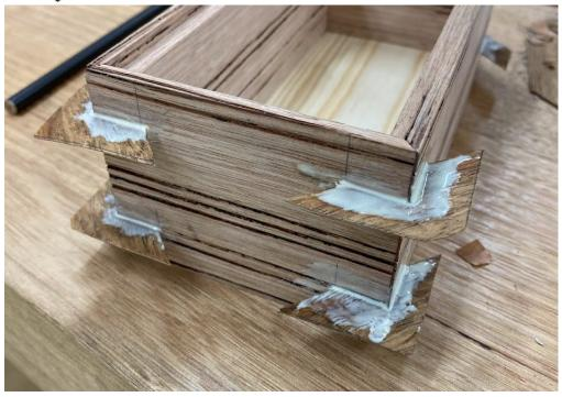
Once dried, with a sharp chisel, pair away the excess veneer from the box. Clamp the box using your workbench vice and pair from the corner into the centre of the box side so that you have supported grain to prevent tear out.
