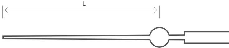
Sweeps are measured from the center fixing hole to the longest tip of each sweep.
