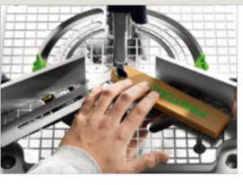
Couldn't be easier – use the bevel to record the angle from the wall or recess, transfer it to the stop system and make the cut.
